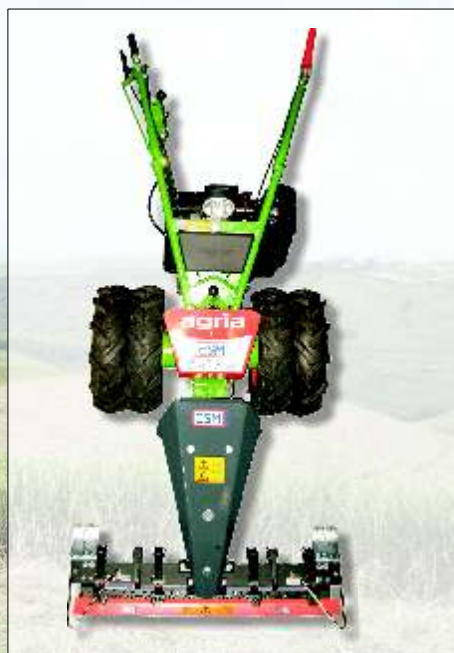
single tyres, standard CaneThumper execution for usage in flat and light slopy areas
