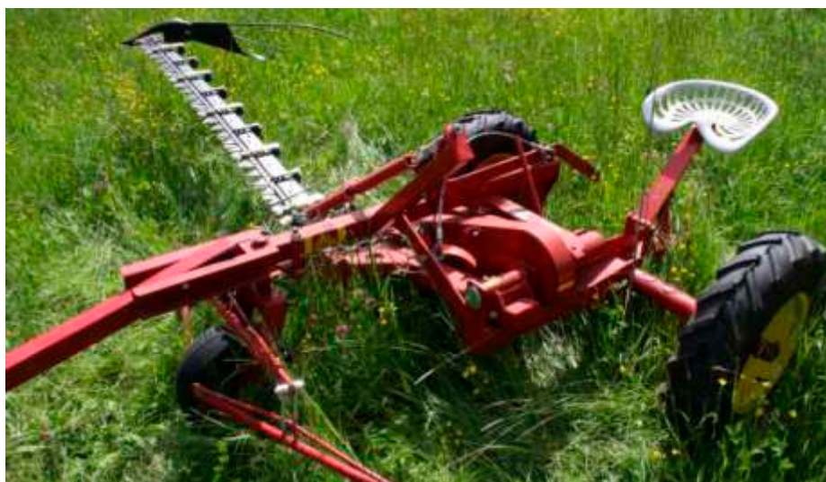
Figure 1: Mower with double knives: advanced technology, cutter bar is 2,2 m long, a three v-belts actuate the chain, very robust, does not plug up, best adapted for mowing meadows with horses, costs: about 6,800 € (Hohegger, Mayer, 2014) TE Sustainable regions (reviewed) Oral 2 RAMIRAN 2015 – 16th International Conference Rural-Urban Symbiosis, 8th – 10th September 2015, Hamburg, Germany
