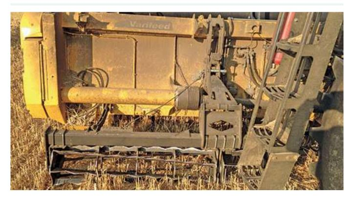
The secondary cutterbar is a self-sharpening, flexible knife usually used for reed-cutting on ditch-clearing excavator buckets. In work it floats on two cage-rollers on the outer extremities of the header and miniskids in the centre section.
