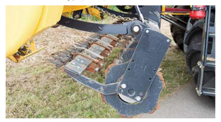
With the wheels rolling in the double-cut straw and the straw chopper providing a downward blast, Mr Ward believes there isn't the requirement for a central roller.
