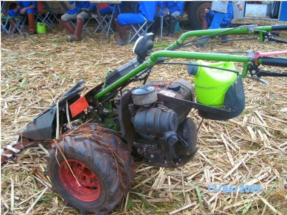
Ready to cut with water bottle and clearing knives attached...
