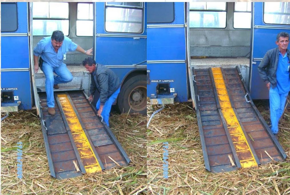
Pulling the ramp out and then ready for loading.
